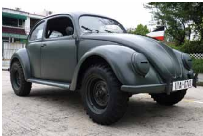
Wider fenders and running boards are distinguishing characteristics of the Type 87/877.
