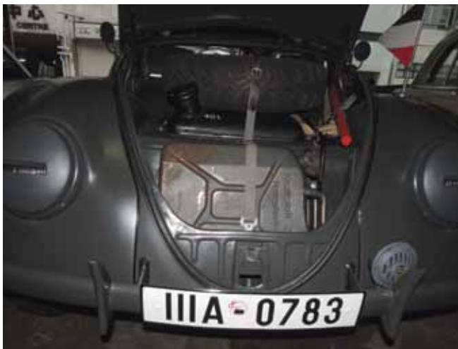
Like a normal wartime Beetle, the 1941 Type 877 prototype carried a spare tire, 20-liter fuel gas can, rear air filter and twin puller set under the front hood. These items are all original to Victor's vehicle.
