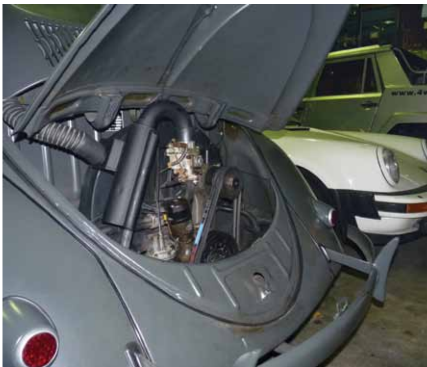
The 986 cubic centimeter, horizontally opposed, four-cylinder, air-cooled engine produced about 23.5 horsepower at 3,000 rpm. Despite excellent performance, only a handful of the four-wheel-drive Kommandeurswagen were built.
